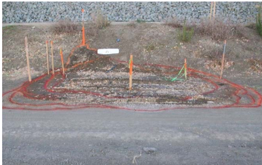
Figure 7. Example of a seepage area showing monitoring efforts and how the limits of a wetted seepage area have varied over time.
