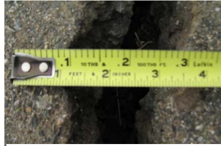
Figure 27. Tension crack monitoring.
