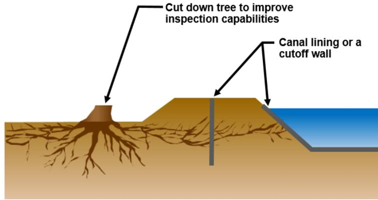
Figure 21. Acceptable methods to cutoff root systems.
