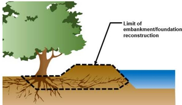
Figure 20. Example of embankment/foundation reconstruction limits.
