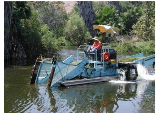
Figure 24. Combination hydrocutter and harvester.
